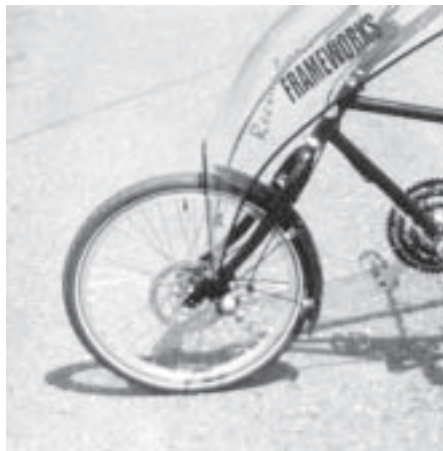
The Cambie accessories all worked wonderfully. Note the fenders, fairing and front disc brake
